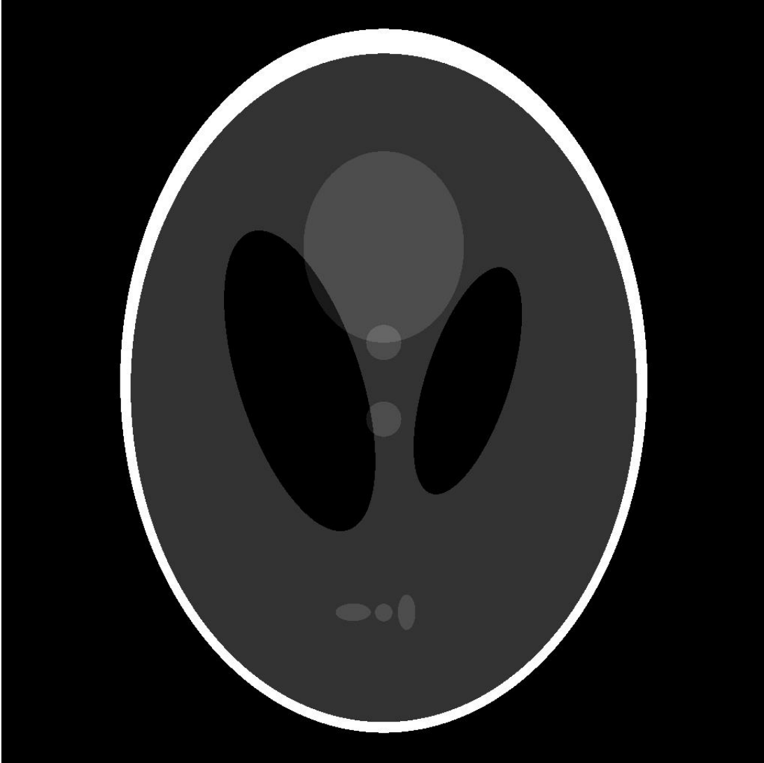
Figure 3: The Shepp-Logan phantom - The standard phantom in the world of image reconstruction.
